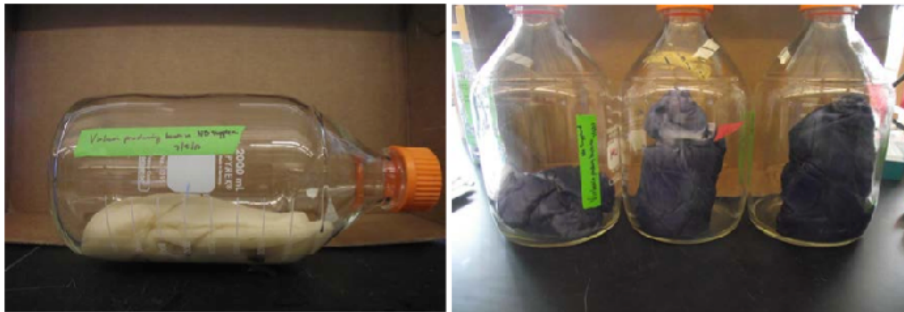
Figure 2: Violacein optimization. 1% Glycerol and 250µM L-tryptophan were added to the nutrient broth media to enhance pigment development. Cotton mats were used to allow bacteria to become sessile and produce violacein faster than with liquid cultures.
